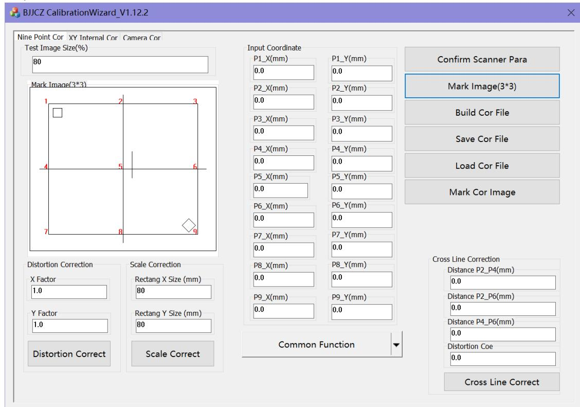
2. Click “Confirm Scanner Para” button, on the popup window click “Making Test Image (3\*3)” button, check the marking result, click “Change Image Type” button to make the software mark image is same as the real marking result. Click “Enter/Exit” button to confirm.
