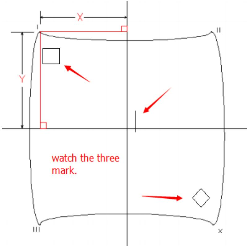
4. Check the X and Y coordinates value if correct, then click "Build 9 Point Cor File" button, then click "Save Cor File" button to save the cor file. Click "Load Cor File" button to load the cor file.
