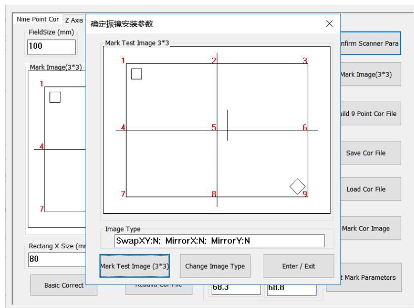
3. Click "Mark Image (3\*3)" button to mark. Measure point 1 to point 9 's coordinate, input the value to software (only input the value, no need to input + or -). (below is point 1's X and Y coordinate)
